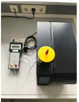
4. <u>Electrostatic charge and potential</u> measured with an electrostatic field meter.
