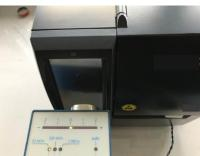
Only the plastics inside the printer are chargeable, but the existing electrostatic fields are shielded by the housing of the printer.
